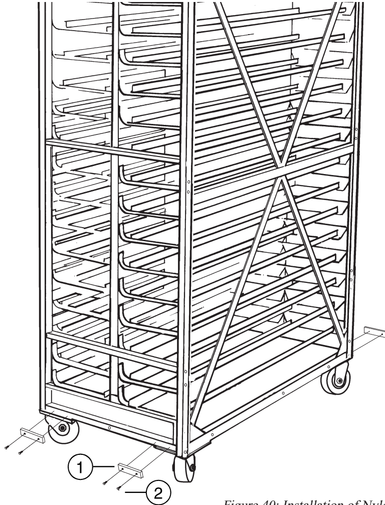
Figure 40: Installation of Nylon Bumpers
